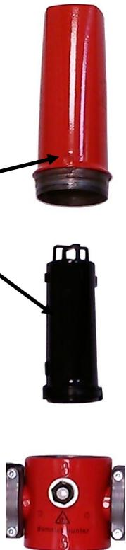
2. Inside the top half bowl should be the ozone filter which is black in colour. This can simply be pulled out with a small amount of pressure.
